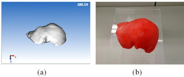
Fig.1 (a) A polyhedral liver with STL format, (b) its 3D printed plastic liver.
