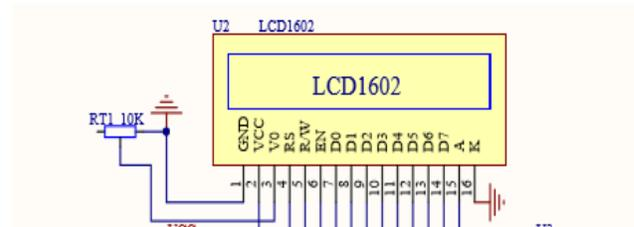
Fig.5. LCD1602 pin diagram
