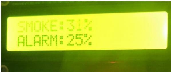
Fig.11. LCD1602 displays when there is smoke
