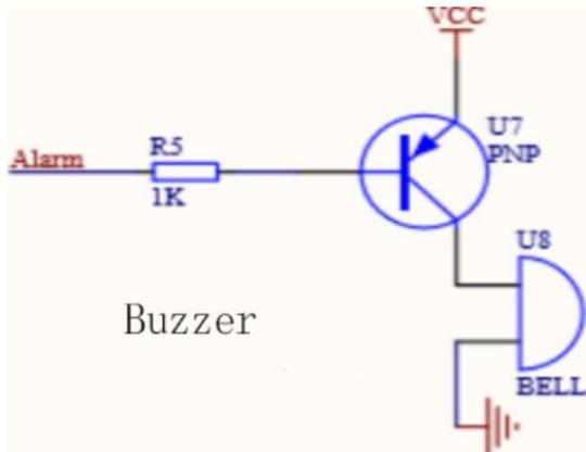
Fig.4. Alarm circuit diagram
