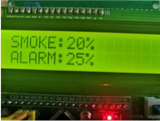
Fig.10. LCD1602 display when there is no smoke
