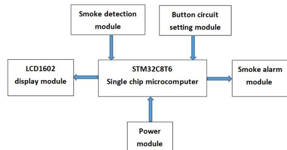
Fig.1. The hardware system structure diagram
