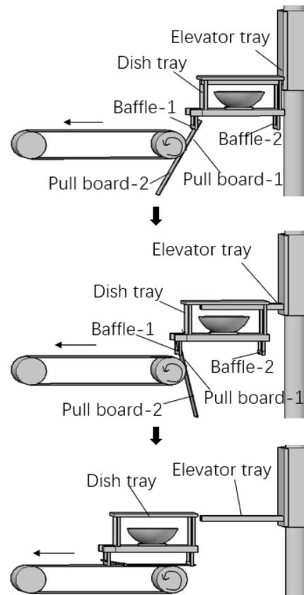
Fig.3. Design of pull board
