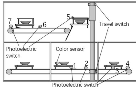
Fig.5. Sensor installation location diagram
