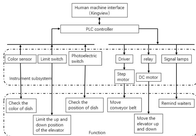
Fig.4. The general framework of automation control system
