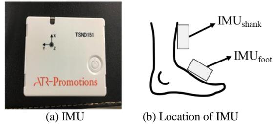
Fig. 3 Photos of the actual IMU(a) and where it was located(b).
