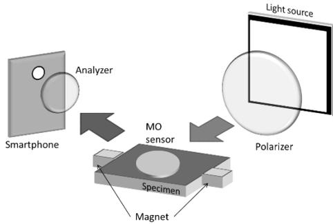
Fig. 2 Schematic diagram of the MO imaging optical system II. (In the case of the low-remnance and the high-remnance elements)
