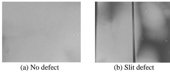
Fig.8 MO images for no defect and slit defect with high spatial resolution MO element
