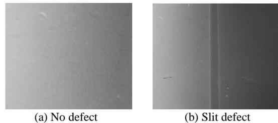
Fig.7 MO images for no defect and slit defect with high spatial resolution MO element
