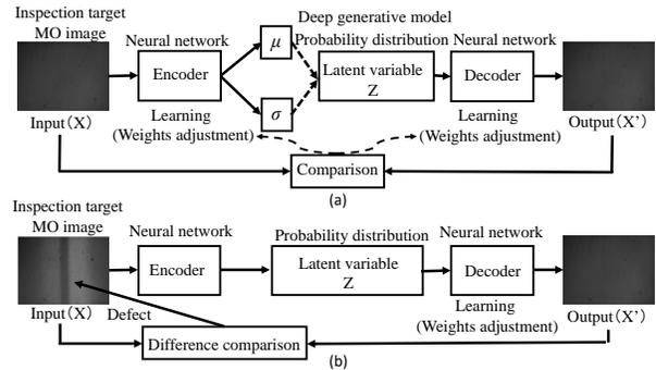
Fig. 4 Learning with the variational autoencoder and detection of anomaly in MO image
