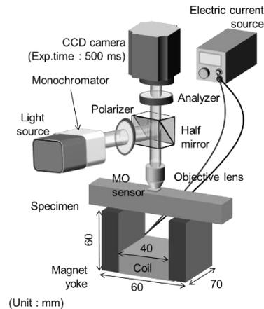
Fig. 1 Schematic diagram of the MO imaging optical system I. (For capturing the high spatial resolution element)
