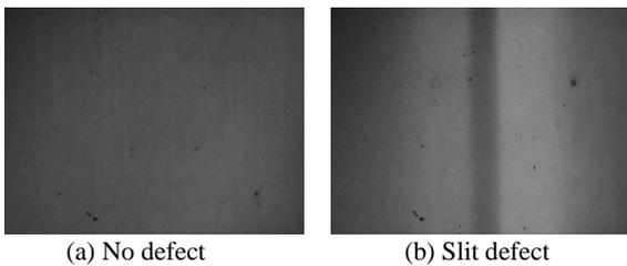
Fig.6 MO images for no defect and slit defect with high spatial resolution MO element
