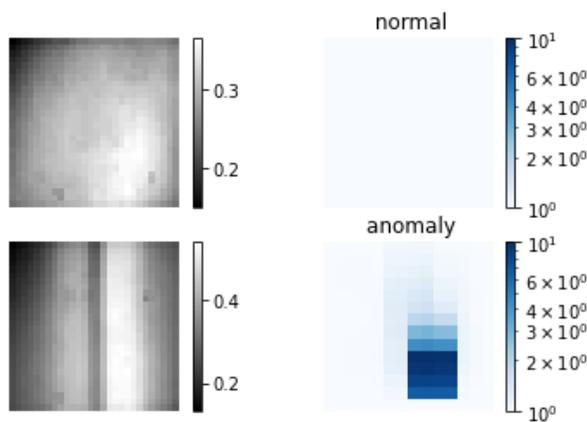
Fig.9 Anomaly heat map for high spatial resolution MO imaging
